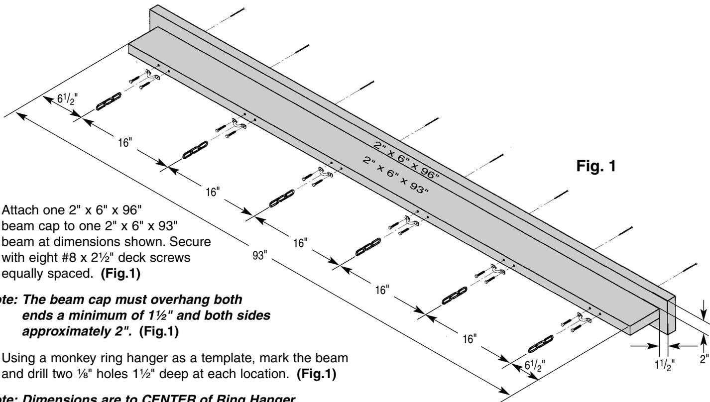
1. Attach one 2" x 6" x 96" beam cap to one 2" x 6" x 93" beam at dimensions shown. Secure with eight #8 x 2½" deck screws equally spaced. (Fig.1)
