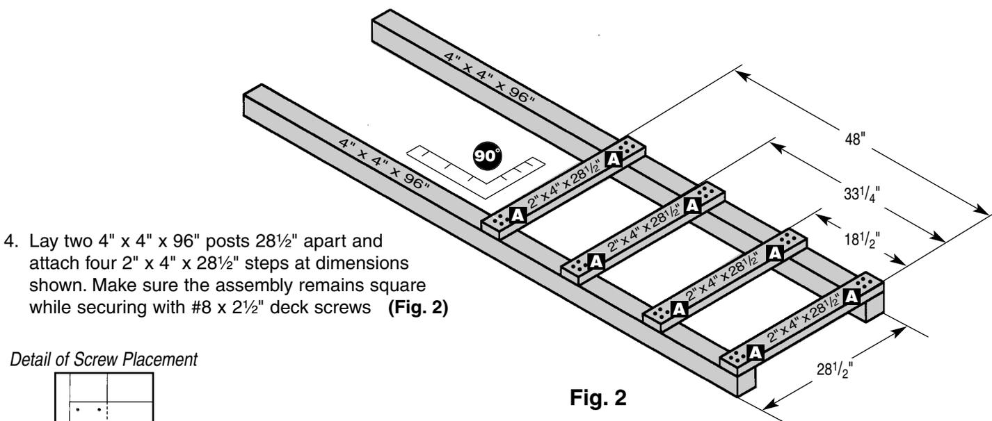
4. Lay two 4" x 4" x 96" posts 28½" apart and attach four 2" x 4" x 28½" steps at dimensions shown. Make sure the assembly remains square while securing with #8 x 2½" deck screws (Fig. 2)
